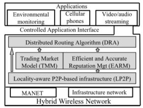
fig 1: A high-level view of the MDR mechanism
